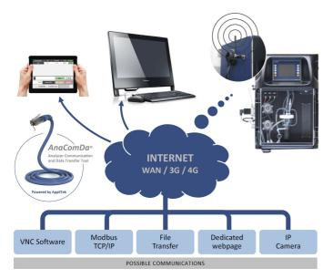
The **AnaComDa®** tool allows to create a secure VPN connection to mobile networks (3G, 4G) or Wide Area Networks, giving authorized users the possibility to use e.g. Modbus TCP/IP control through a dedicated webpage or via VNC software. The tool also allows extended data logging in the cloud and visualization (connection of an IP camera). With the VPN created, FTP protocols can be used directly from a PC or a mobile device.
